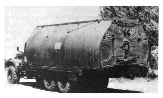
Figure 6-50. PMP heavy folding bridge. This new-type "ribbon bridge" provides a rapid-assembly heavy (class 60) bridge. The sections are carried folded on the backs of trucks. The trucks back up to the water's edge and dump their spans which open automatically as they hit the water. The bridge is assembled in the water along the shoreline and positioned by power boats.
